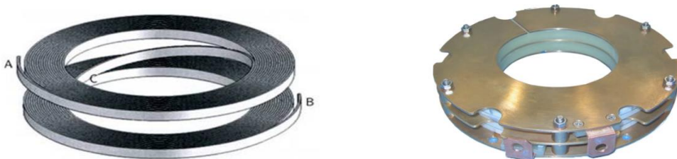
Figure 10 a) The concept of double pancake b) Double pancake manufactured by HTS110
