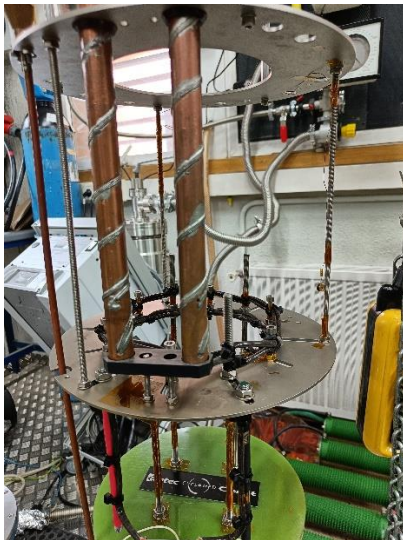
Figure 34 PK0 coil being tested in a cryostat in CIEMAT facilities (left) and picture during LHe testing of PK0 coil (right)
