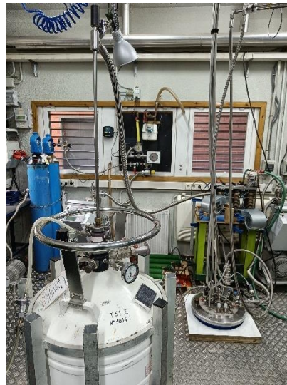
Figure 34 PK0 coil being tested in a cryostat in CIEMAT facilities (left) and picture during LHe testing of PK0 coil (right)
